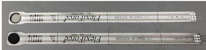
Figure 6.1. Selected force sensor top view, bumper added on bottom sensor
