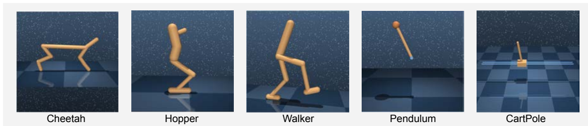
Figure 4.11: Visualization of various tasks in DeepMind Control Suite. DeepMind Control Suite includes image-based control tasks with physics simulation. We mainly experiment on locomotion tasks in this environment.
