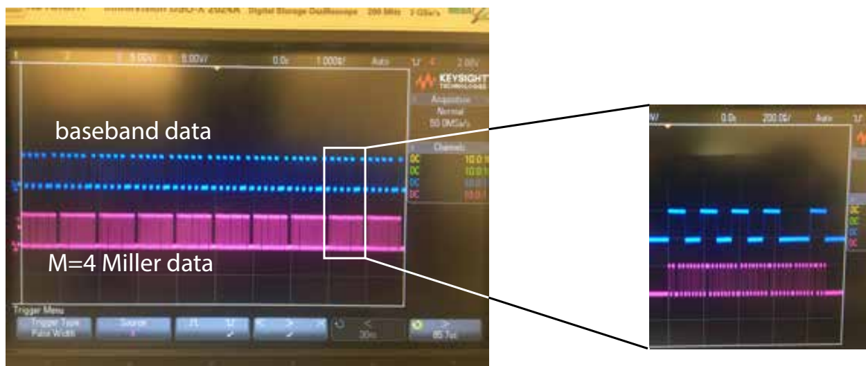
Figure 4.21: Oscilloscope measurement of Miller encoding using ATtiny20 microcontroller.
