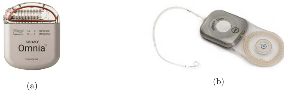
Figure 2.6: Examples of implanted medical devices utilizing wire-wound coils (WWC) for inductive charging. Images courtesy of Nevro and Advanced Bionics [34, 35].
