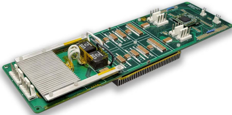
Figure 1.1: High power density 7 kW dual-interleaved 6-level FCML inverter / rectifier hardware prototype.
