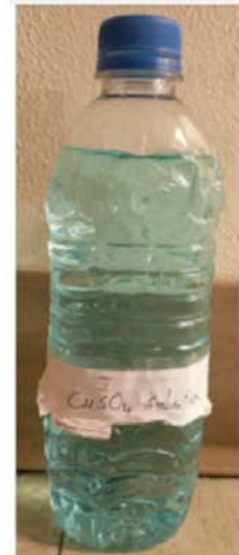
Figure 3.4: Shim array placement and bottle phantom. The far left is the RF solenoid and its sleeve (cover removed). The B_0 field direction is to the right, while the B_1 field direction is out of the bore. The placement of the shim array on top of the RF solenoid is shown in the middle. On the right is a copper sulfate doped bottle phantom, inserted into the solenoid shown on the far left.
