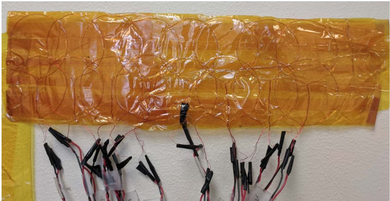
Figure 4.1: The second iteration of our shim array, made with 32-gauge magnet wire. This is wrapped around the RF solenoid when scanning.
