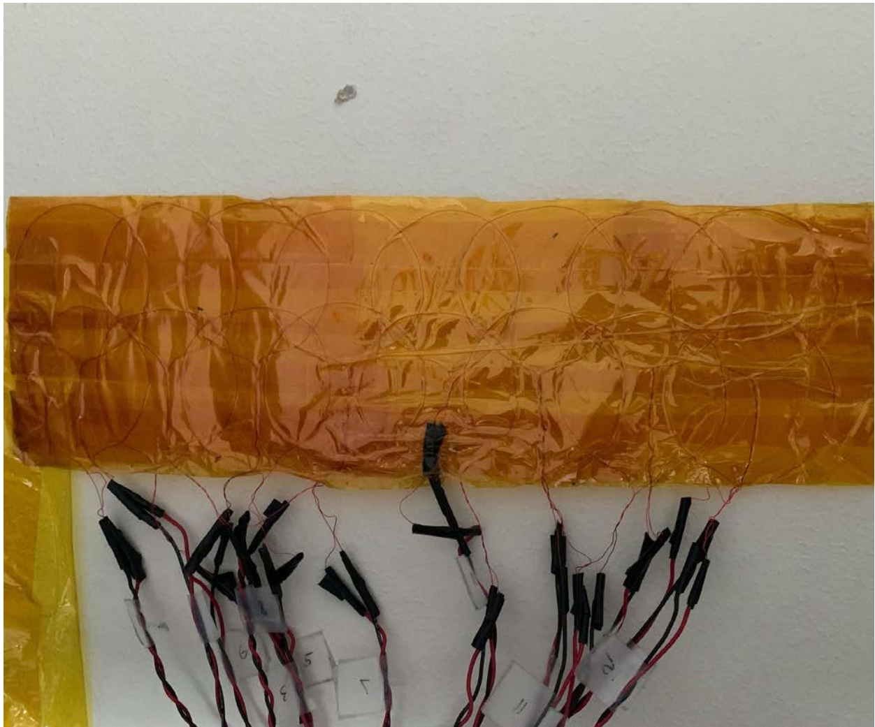
Figure 4.4: Version 2 of the local shim array. Constructed on kapton tape using 32 gauge copper magnet wire. Connected to improved current driver system as shown in Figure 4.2. Lessened the coupling problem associated with the wide copper tape.
