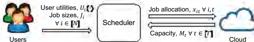
Figure 9.2: A block diagram schematic of the system with N users and T service tiers
