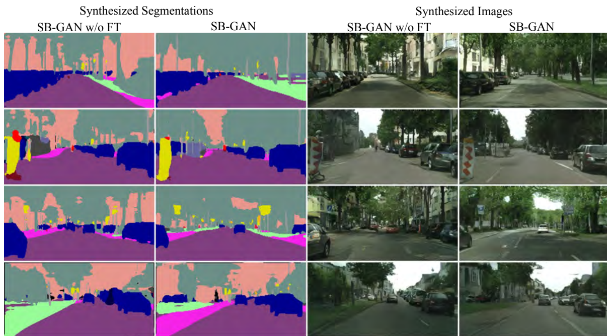
Figure 3.8: The effect of fine-tuning on the baseline setup for the Cityscapes-25K dataset. We observe improvements in both the global structure of the segmentations and the performance of semantic image synthesis, resulting in images of higher quality.
