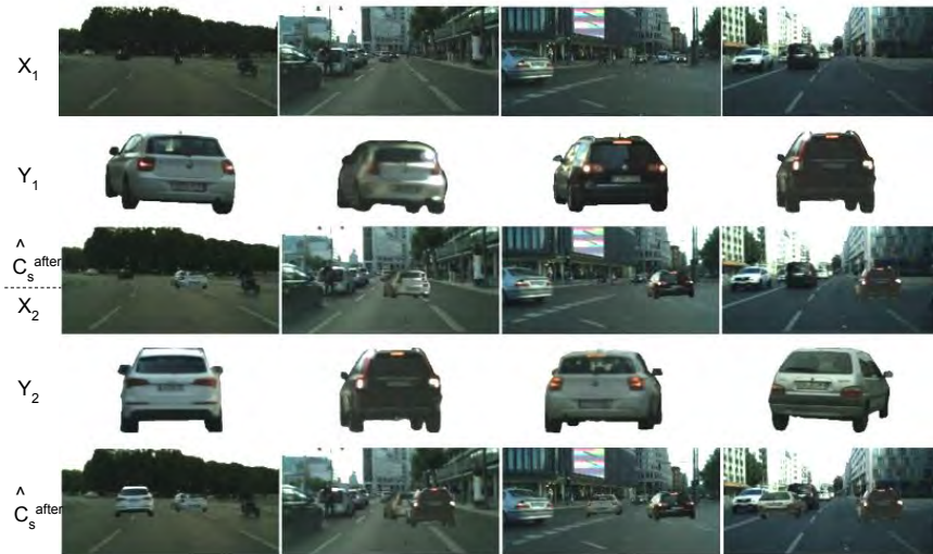
Figure 4.10: Test examples for an iterative extension of the street scenes-cars composition task to more than two objects. The first two rows show the input street and the input car images in the first iteration. The 3rd row illustrates the output of our compositional generator, used as the street scene inputs for the next iteration to be composed with the cars shown in the 4th row. The 5th row indicates the final generated composite image of the two cars added to the street scenes iteratively.
