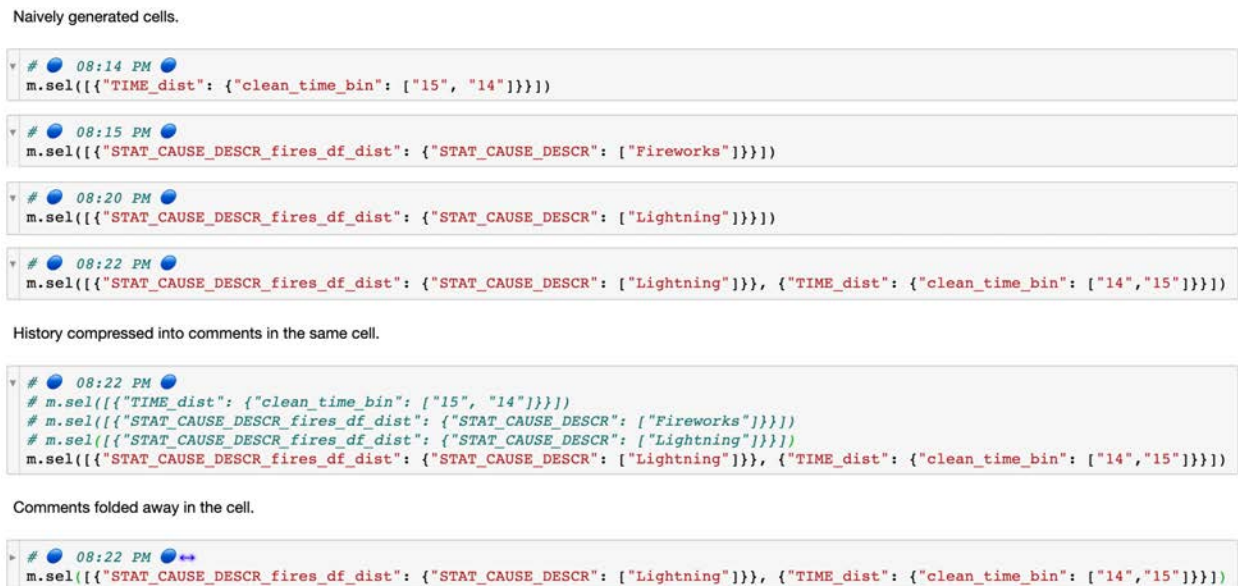
Figure 4.6: A demonstration of three designs of selection cells. The top four cells represent the result of creating new cells every time there is an interaction. The second last cell represents all four selections, with three commented out. The last cell represents the previous cell folded, and is the design we finalized on for B2.
