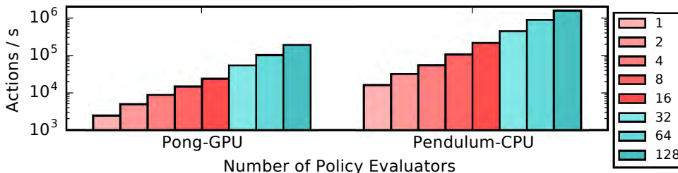
Figure 3.7: Policy evaluation throughput scales nearly linearly from 1 to 128 cores. PongNoFrameskip-v4 on GPU scales from 2.4k to \sim 200k actions/s, and Pendulum-v0 on CPU from 15k to 1.5M actions/s. We use a single p3.16xl AWS instance to evaluate from 1-16 cores, and a cluster of four p3.16xl instances from 32-128 cores, spreading actors evenly across the cluster. Rollout workers (evaluators) compute actions for 64 agents at a time, and share the GPUs on the machine.
