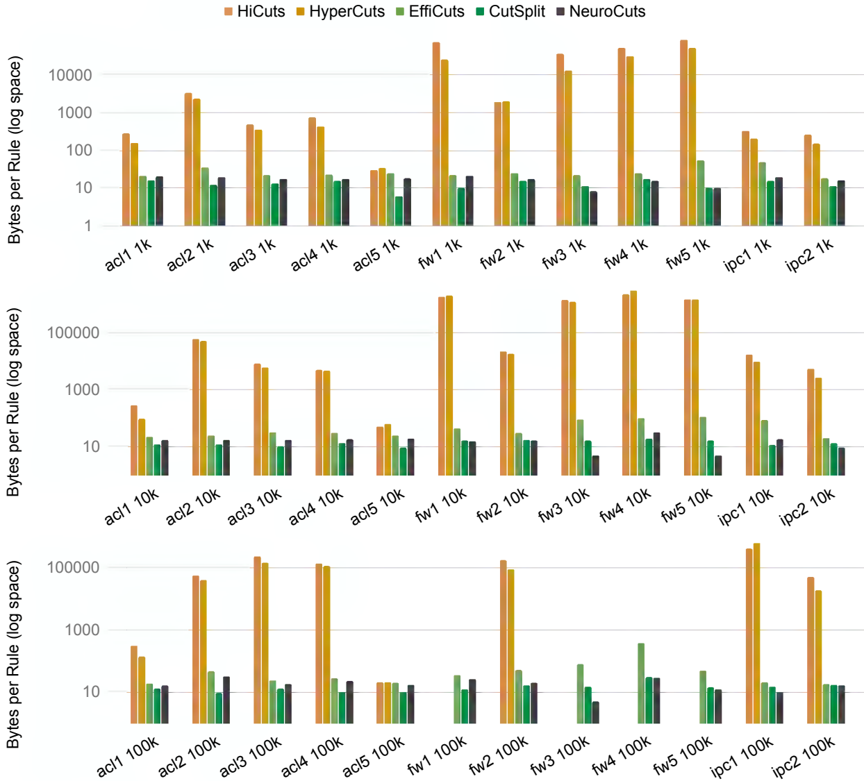
Figure 5.9: Memory footprint (bytes per rule) used for HiCuts, HyperCuts, EffiCuts, and NeuroCuts (space-optimized) across the (1k, 10k, and 100k) sized rulesets. We omit four entries for HiCuts and HyperCuts that did not complete after more than 24 hours.
