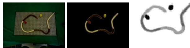
Figure 5.8: Preprocessing procedure. Image 1: original photo as seen by the PR2, Image 2: background removed from image, Image 3: Preprocessed to have one color channel
