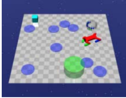
Figure 8.2: Rendering from the DOGGOGOAL1 environment from Safety Gym. The red, four-legged robot must walk to the green cylinder while avoiding other objects, and receives coarse egocentric sensor readings of their locations.
