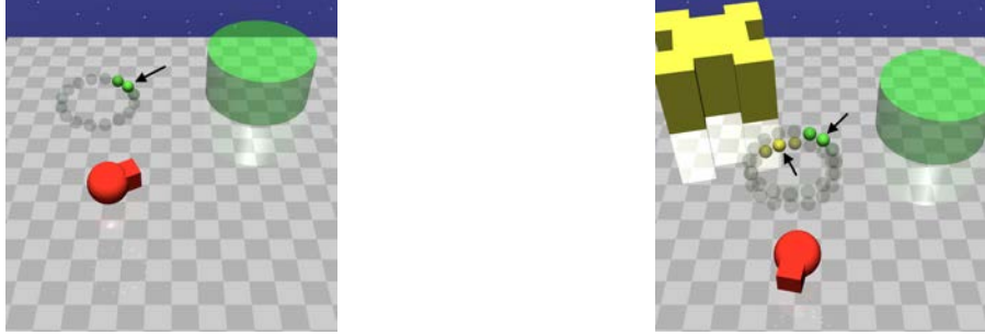
Figure 7.4: Visualizations of pseudo-lidar observation spaces. On the left, we see a lidar halo representing the goal pseudo-lidar for this agent. On the right, we see lidar halos representing the goal pseudo-lidar and the box pseudo-lidar.
