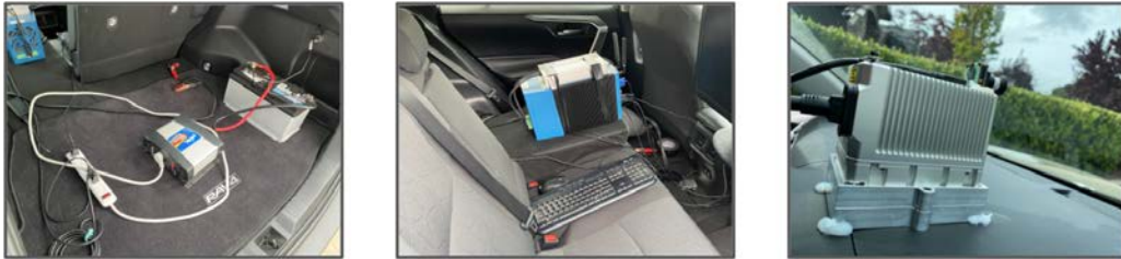
Figure 9: Data collection hardware setup. Left: Power supply configuration. Middle: Computer and monitor. Right: LiDAR and camera.
