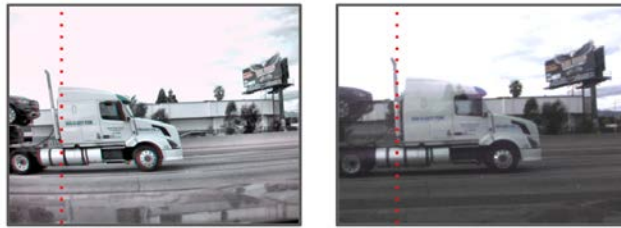
Figure 11: Rolling vs global shutter. Left: Image from traditional rolling shutter camera. Right: Image from the global shutter camera used in TODD. The dotted red line represents the true vertical axis.
