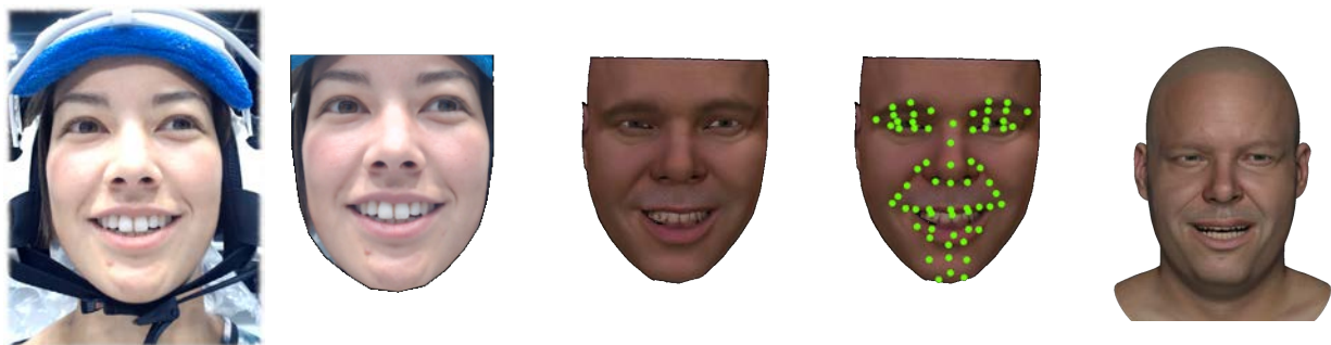
Figure 6.1: Visualization of the full blendweight solving process. Starting with a frame from a recorded video on the left, we employ style transfer to produce the middle image that has the appearance of the blendshape model but preserves the expression of the actor in the recorded frame. We then apply our blendweight optimization method to produce the deformed facial model shown on the right.
