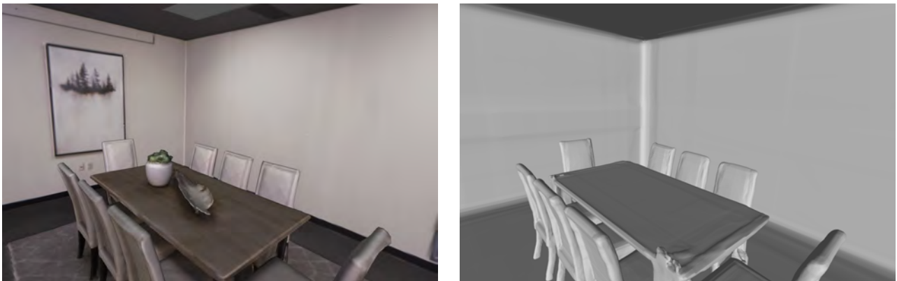
Figure 4.11: Sample results from using the methods proposed in the chapter to model the layout and objects in an indoor scene. Left: 3D scan of an input scene, Right: model generated by our proposed methods.
