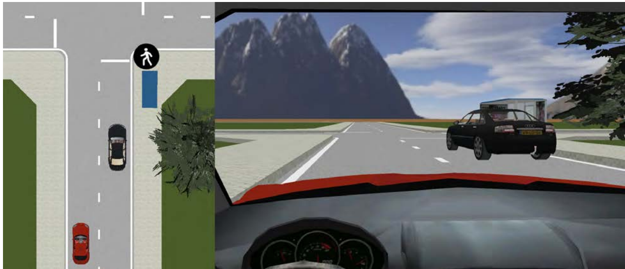
Figure 2.1: Motivating example of occluded pedestrian. ( Left ) Topview showing the red ego vehicle, the black car causing occlusion, and the hidden pedestrian. We model the actions of the black car as sensor inputs. ( Right ) Viewpoint from the red car (ego vehicle), showing that the pedestrian is occluded.
