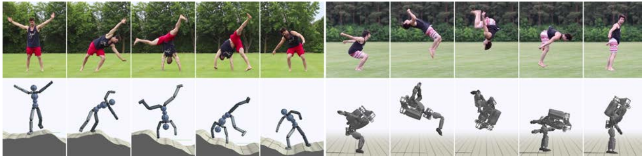
Figure 4.1: Simulated characters performing highly dynamic skills learned by imitating video clips of human demonstrations. Left: Humanoid performing cartwheel B on irregular terrain. Right: Backflip A retargeted to a simulated Atlas robot. (Video 1 )
