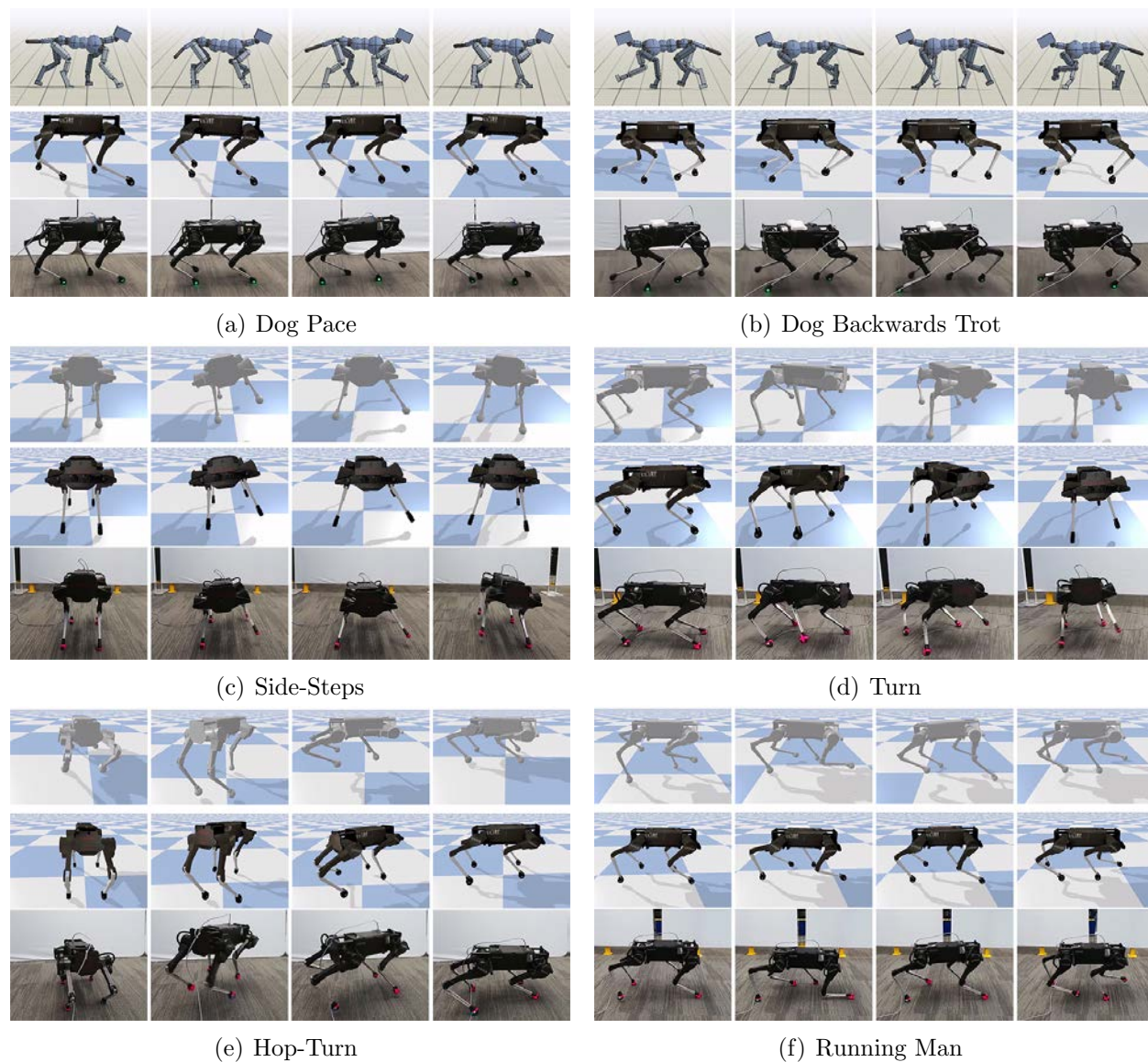
Figure 10.4: Laikago robot performing skills learned by imitating reference motions. Top: Reference motion. Middle: Simulated robot. Bottom: Real robot.
