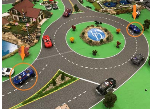
Figure 3.7: Experiment with two platoons being led by RL vehicles (blue, circled).
