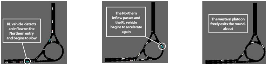
Figure 4.3: Two RL-controlled AVs trained with adversarial multi-agent noise demonstrate emergent ramp metering behavior.
