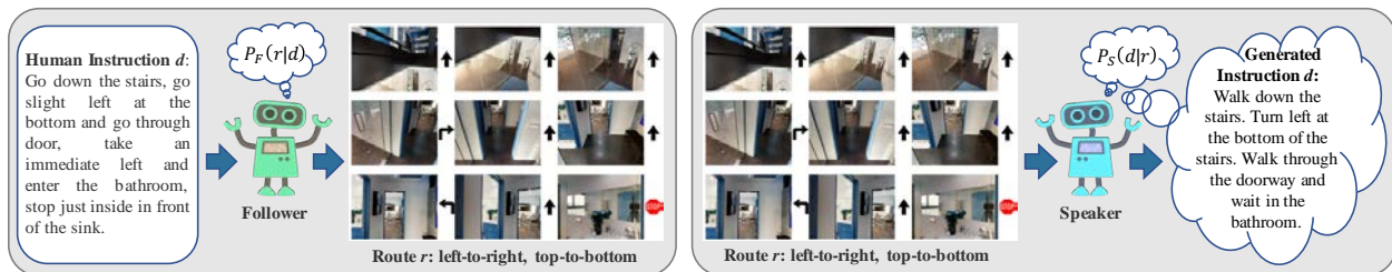
Figure 3.1: The task of vision-and-language navigation is to perform a sequence of actions (navigate through the environment) according to human natural language instructions. Our approach consists of an instruction follower model (left) and a speaker model (right).
