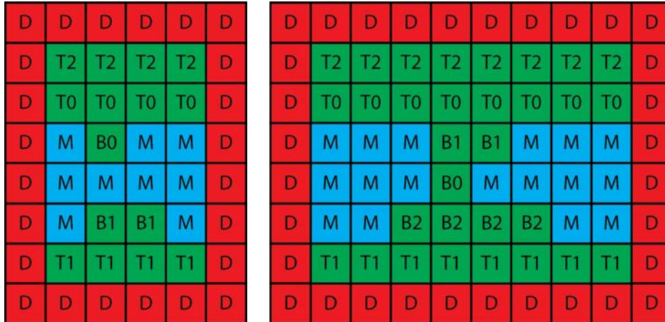
Figure 3.25: PI IDAC patterns with different number of bits and bias rows
