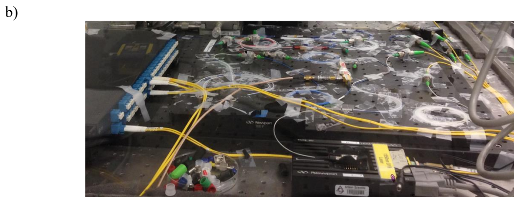
Figure 5.1: a) Schematic of fiber-based interferometry setup. PM is a phase modulator, and DAQ is a data acquisition board. b) A photograph of our fiber-based demultiplexed multiwavelength interferometry setup on a floating optical table. Tapes were used to secure the fibers to the table to stabilize micromovements of the fiber.
