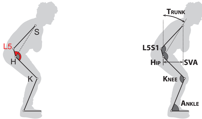
Figure 2.3: Left: Model used for L5S1 angle estimation. The sagittal location of the shoulder, L5S1, hip, and knee are shown. The included angle at the hip is used to predict the angle at L5S1. Right: sagittal plane model. Joint centers and angle definitions are shown. The definition of the Sagittal Vertical Axis (SVA) metric is also shown.
