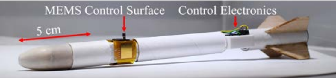
Figure 3.3: The fully assembled rocket, consisting of a MEMS control surface and its 2x4 mm2 steel airfoil, a single-cell LiPo battery, and control electronics.
