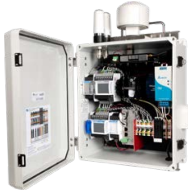
Figure 5: The \mu PMU sensor holds the promise of increased distribution network visibility. The white “mushroom” on top of the device box is an antenna for receiving the GPS clock signal.
