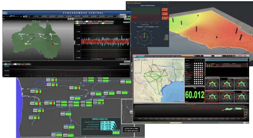
Figure 14: Interfaces of industry tools for oscillation monitoring. Clockwise from top left: SEL, Space-Time Insight [99], ERCOT [97], BPA [98]
