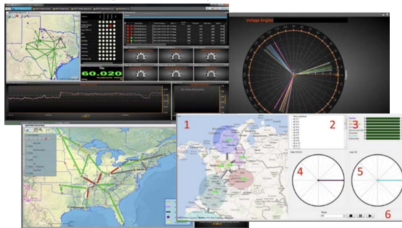
Figure 15: Interfaces of industry tools for angle difference monitoring. Clockwise from top left: ERCOT, Dominion, Columbia WAMS, and EPG [100]
