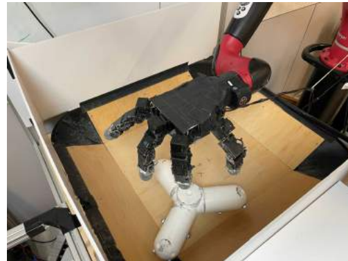
Figure 14.5: Real-world hand-arm manipulation platform. The system comprises a 16 DoF hand mounted on a 6 DoF Sawyer arm. The goal of the task is to perform in-hand reorientation, as illustrated in Fig 14.10 or pipe insertion as shown in Fig 14.11
