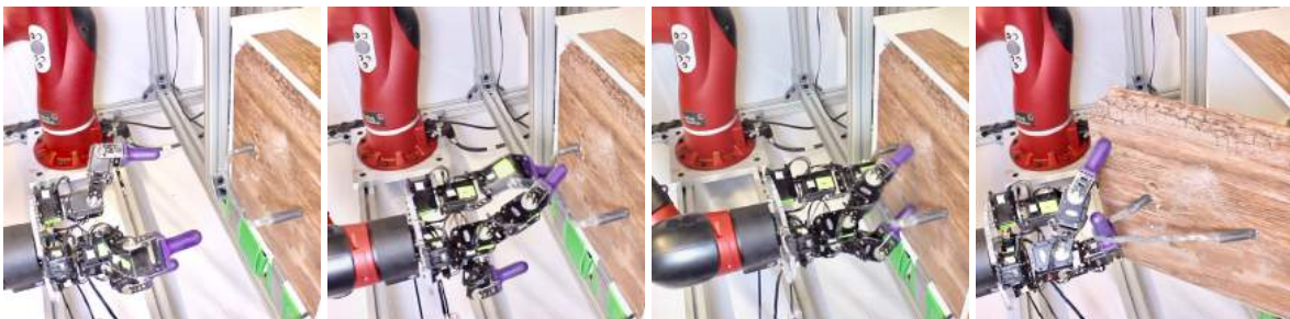
Figure 9.9: Visualization of a policy that has learned to open a door after 16 hours of training. The robot learns to move towards the door, grasp the deformable handle, and then pull the door open.
