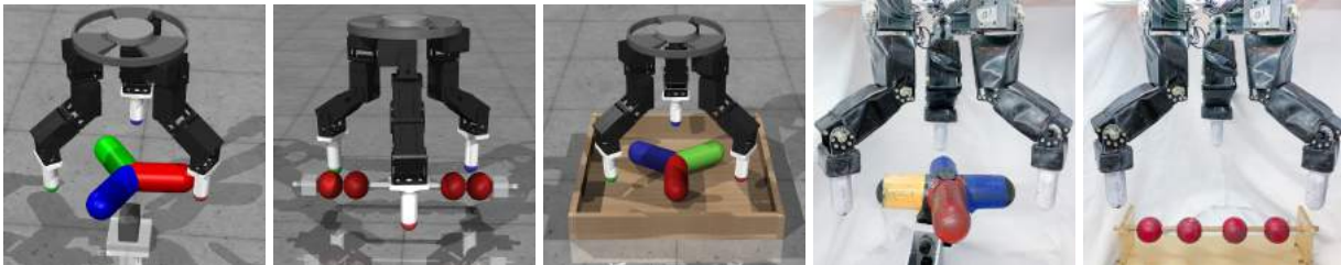
Figure 13.6: Visualizations of the goal configurations of the simulated and real world tasks being considered. From left to right we depict valve rotation, bead manipulation and free object repositioning in simulation, as well as valve rotation and bead manipulation manipulation in the real world.
