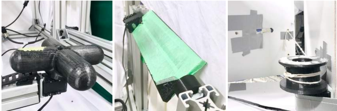
Figure 9.6: Dynamixel driven sensing and reset mechanisms. Left to Right: rigid valve, box, door.
