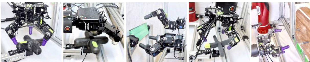
Figure 9.1: We demonstrate that DRL can learn a wide range of dexterous manipulation skills with multi-fingered hands, such as opening door with flexible handle, rotating a cross-shaped valve, and rotating the same valve but with a deformable foam handle, which presents an additional physical challenge, and box flipping.
