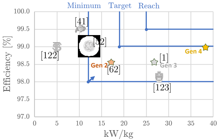
(a) Comparison of this work (Gen 4) performance against NASA electric aircraft targets [24] and competing designs.
