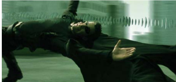
Figure 1 b): For the bullet time scene in "The Matrix", the VFX team realized they didn't have enough frames for smooth motion. They ran an optical flow pass to track where the pixels moved between adjacent frames, and created "smears" using the vectors from optical flow for interpolated, smoothed out motion [15].
