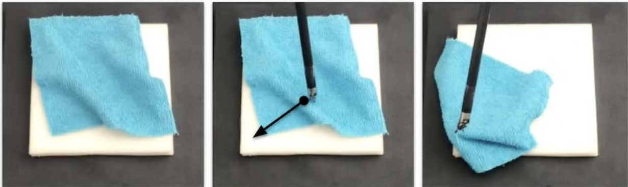
Figure 3.7: A poor action from a policy trained on only depth images. Given the situation shown in the left image, the learned policy erroneously picks a point near the center of the fabric. The resulting pick, followed by the pull to the lower left, causes a major decrease in coverage and makes it hard for the robot to recover.
