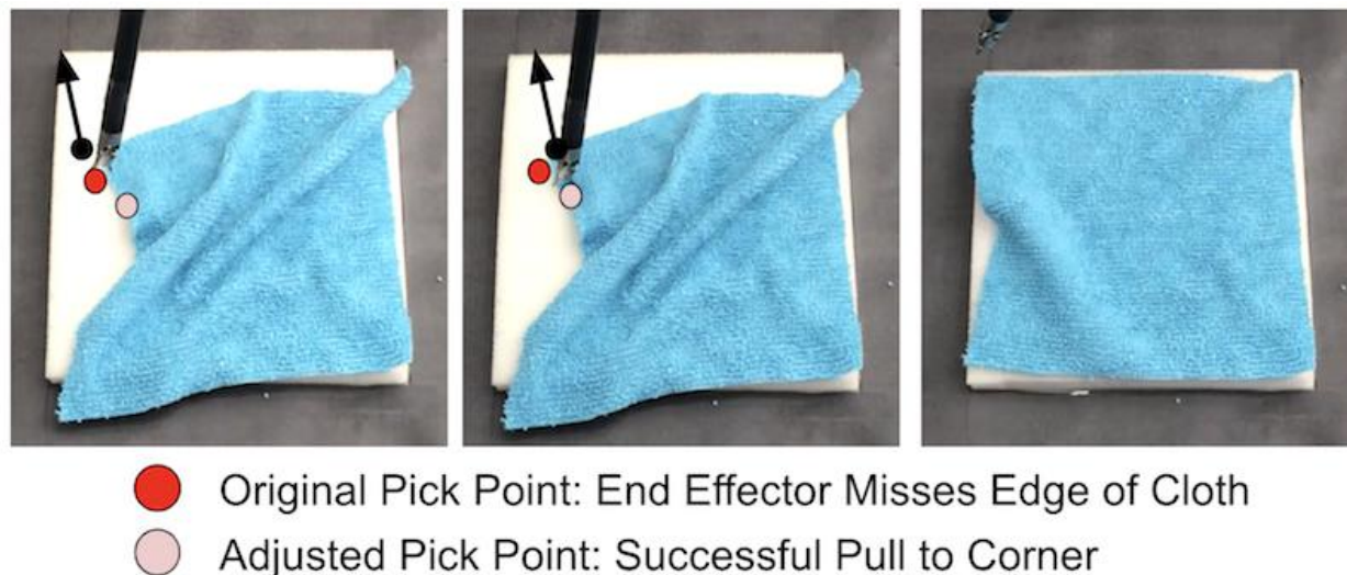
Figure B.1: Correcting the dVRK when it slightly misses fabric. Left: the dVRK executes a pick point (indicated with the red circle) but barely misses the fabric. Middle: it detects that the fabric has not changed, and the resulting action is constrained to be closer to the center and touches the fabric (light pink circle). Right: the pull vector results in high coverage.
