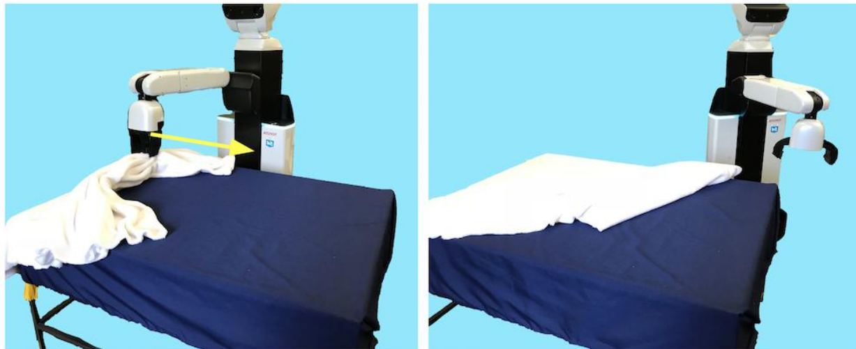
Figure 2.10: The HSR following the analytic baseline. It grasps at the highest reachable point and pulls in the direction of the yellow arrow, improving coverage.
