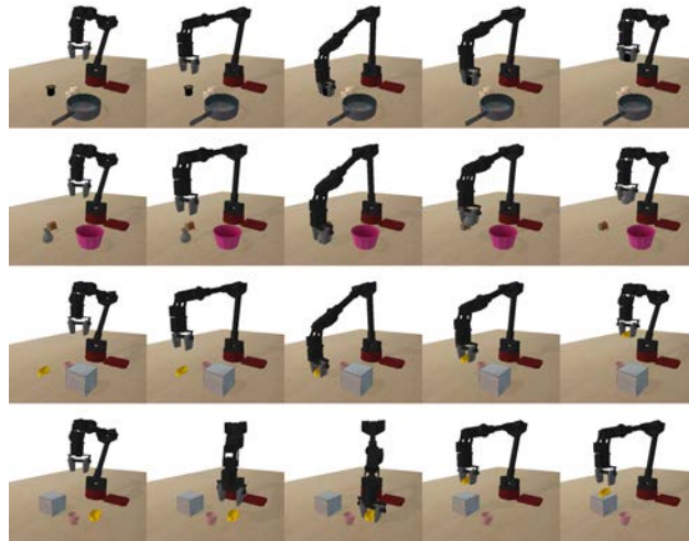
Figure C.3: In the first row, the objective is to grasp a can and lift it above a certain height. Rows two and three are similar, except the objective is to grasp a vase and a baseball cap, respectively. The final row depicts a task where the goal is to pick the baseball cap and place it on the marble cube.
