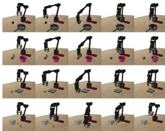
Figure 4.3: Tasks. A subset of our evaluation tasks, with one task shown in each row. In the first task (first row), the objective is to pick up a can and place it in the pan. In the second task, the robot must pick up the vase and put it in the basket. In the third task, the goal is to place the chair on top of the checkerboard. In the fourth task, the robot must pick up the mug and hold it above a certain height. Initial positions of all objects are randomized, and must be inferred from visual observations. Not all objects in the scene are relevant to the current task.
