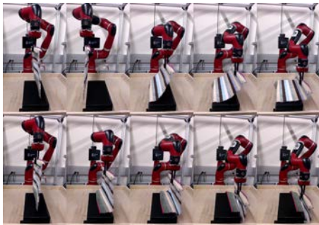
Figure 3.6: In this figure, we demonstrate why learning a reward function on pixels is necessary for solving complex tasks in the real world. The task here is to drape a cloth over a box. The top row shows a rollout from the final policy trained by our method, while the bottom row shows a rollout from a policy trained on a hand-defined reward on robot state alone. Our policy is able to successfully drape the cloth over the box, while the policy trained without vision only sees the end-effector position, which it succeeds in moving to the right place, but fails to drape the cloth on the box.
