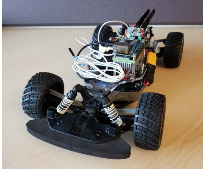
Figure 1.1. As part of an experimental research effort, we have developed a scaled-car test platform for conducting various experiments. We integrated our test vehicle’s hardware based on the f1tenth platform (see https://f1tenth.org/about.html ). The test platform was developed in collaboration with Sirej Dua, Milad Noori, Canberk Hurel, and Nicholas Liu.
