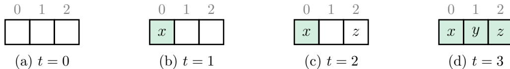
Figure 2.2: At time t = 0 , no state machine commands are chosen. At time t = 1 command x is chosen in slot 0. At times t = 2 and t = 3 , commands z and y are chosen in slots 2 and 1. Executed commands are shaded green. Note that all state machines execute the commands x, y, z in log order.
