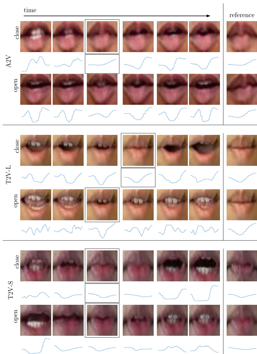
Figure 5.3: Six sequential frames extracted from a single MBP occurrence in different deep-fake videos. Shown on the right is a reference frame where the mouth is clearly closed. Shown below each frame is a 1-D intensity profile used to automatically classify the mouth as open or close. The bounding box corresponds to a frame that matched the reference frame shown to the right (only the closed-mouth sequences match).
