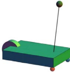
Figure 2: The Chaplygin sleigh model with a moveable mass attached. Here the knife is illustrated as a wheel, but the model is the same as in Figure 1, with the addition of a mass separate from the sleigh body mass which can move in relation to the sleigh body.
