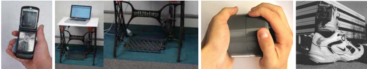
Figure 3: (left to right) Squeeze mobile phone that requires users to squeeze to power it [106]; Treadle laptop table that requires users to pedal to power their laptop [106]; a pair of sneakers with piezoelectric power-generating insoles and a self-powered transmitter [100]
