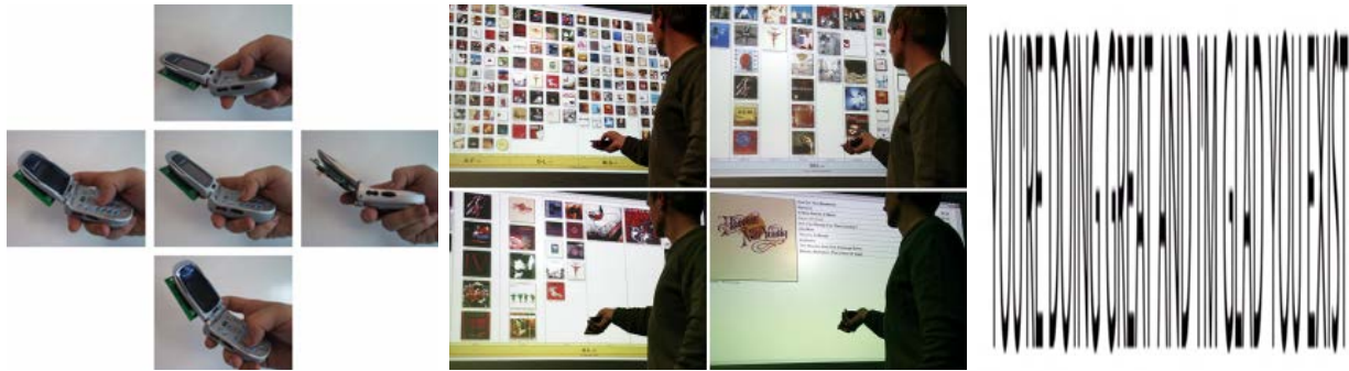
Figure 22: (left to right) TiltText , a system that lets users tilt their mobile phone to indicate characters to type [145]; tilt gestures used to control distant displays [25]; Tilt your phone optical illusion reading “YOU’RE DOING GREAT AND I’M GLAD YOU EXIST” [132]
