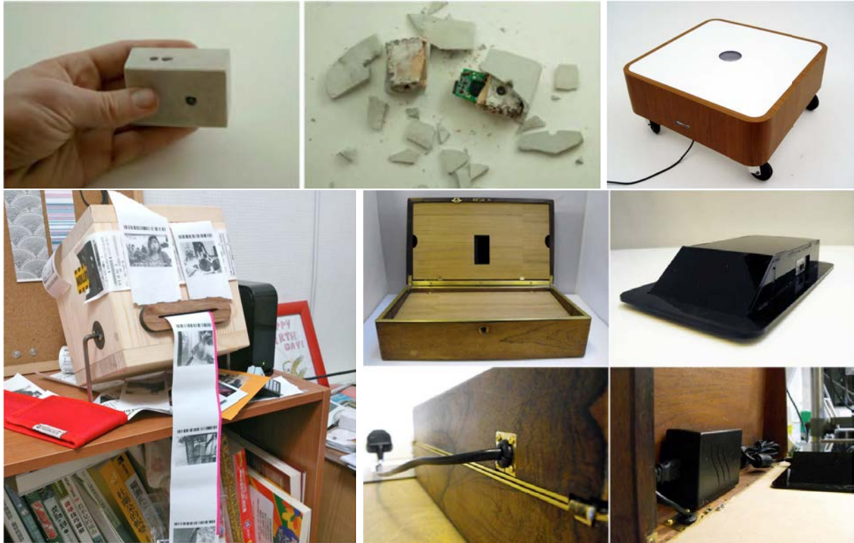
Figure 5: (top row, left to right) Capsule Camera , a counterfunctional digital camera with a concrete enclosure that requires sawing and breaking apart to access the SD card [105]; Drift Table , an interactive coffee table that adjusts qualities of an embedded aerial landscape view based on shifting physical weight on the table [40]. (bottom row, left to right) Reflexive Printer , a physical device that prints one halftone image a day and deletes the corresponding digital copy [133]; Photobox , a domestic device that prints old photographs at random intervals over months [97]
