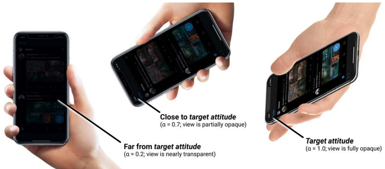
Figure 23: The Tilter iOS mobile application randomly generates a target holding angle that the user must discover and match at various time intervals throughout a session in order to reveal the onscreen display. When the user is far from the target holding angle, the display is dim; when the user tilts the phone closer to the target the display brightens.
