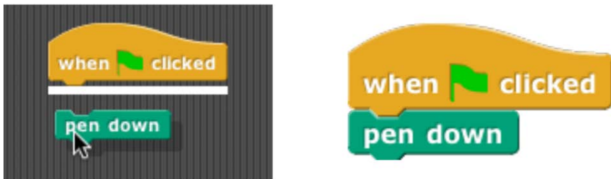
Figure 3.2: Snap! blocks 1 snap together to form executable code-blocks. The yellow block shown above functions as the main function in some programming languages, and the green pen down block lets the sprite start drawing on stage.
