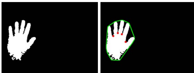
Figure 2.6: Segmented hand and convexity defects
