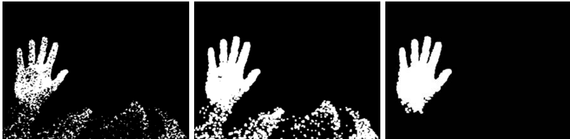
Figure 2.4: Face removal, dilation, and hand segmentation
