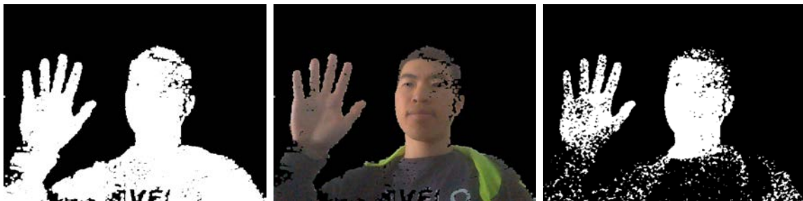
Figure 2.3: Background subtraction, image mask, and color segmentation
