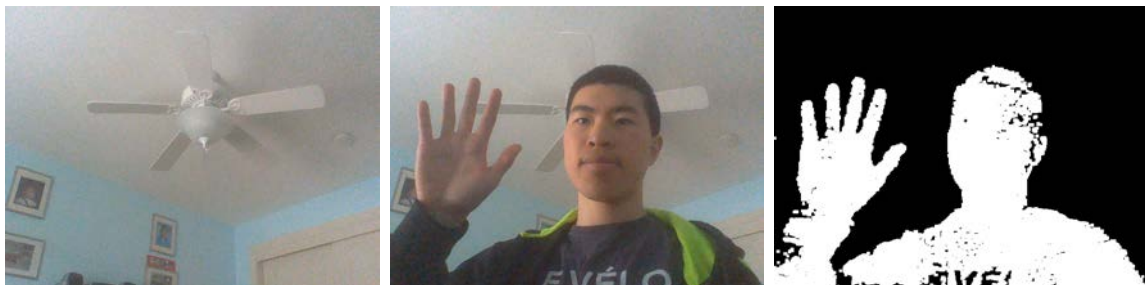
Figure 2.2: Background, captured frame, and background subtraction
