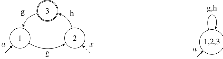
Figure 5.2: Left: The set of solutions to \psi in Example 14. Right: The resulting automaton (without x transition and accepting state) after merging states 1 and 3.
