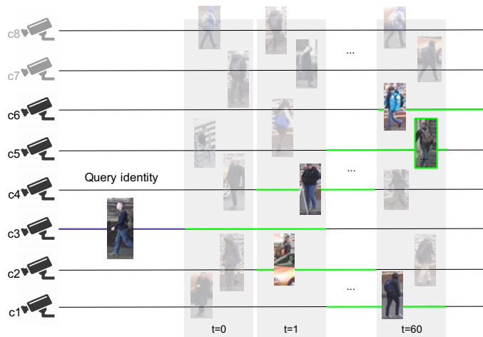
Figure 4.1: ReXCam exploits a learned model of spatial and temporal correlations , built on historical data, to reduce compute workload at inference time. In this figure, the camera network (compressed to 1-D) is represented on the y-axis, and time on the x-axis. In searching for a query identity, ReXCam eliminates some cameras entirely (spatial filtering), and searches the others only within a narrow time window (temporal filtering).
