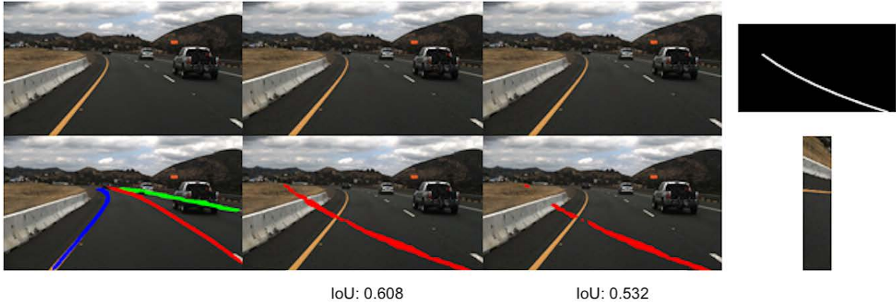
Figure 5. Example of L-infinity bounded attack. From left to right, the vertical pairs of images represent a clean image, a nonadaptive attack, and an adaptive attack against a 3-layer verification model. The second row shows the proposal output by the lane detection model superimposed on the scene, and IoU values below. IoU values are with respect to the target lane binary segmentation map, shown in the upper right, and the resulting stabilized lane is shown below. Under bounded attack, the attacker is able to assert full control over the scene and induce arbitrary lane configurations.
