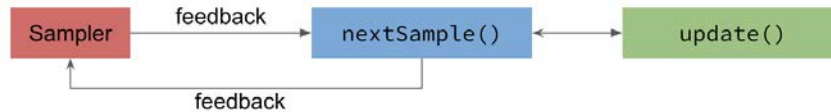
Figure 2.5: Legacy sampling and updating process in active samplers. The nextSample() function is responsible for updating the internal state by calling update() with the most recently generated sample.
