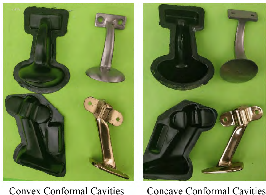
Figure 4.6: Examples of Physical Kitting Cavities: The handrail bracket (bottom) and the ornamental handrail bracket (top), next to the corresponding convex cavity (left) and concave cavity (right).
