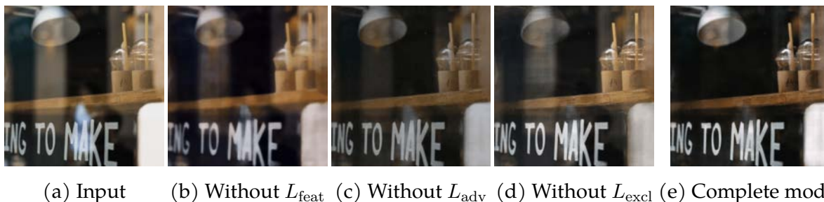
Figure 3.8: Visual comparisons on the three perceptual loss functions, evaluated on a real-world image. In (b), we replace L_{\text{feat}} with image space L^1 loss and observed overly-smooth output. (c) shows artifacts of color degradation and noticeable residuals without L_{\text{adv}} . In (d), the lack of L_{\text{excl}} makes the predicted transmission have undesired reflection residuals. Our complete model in (e) is able to produce better and cleaner prediction.
