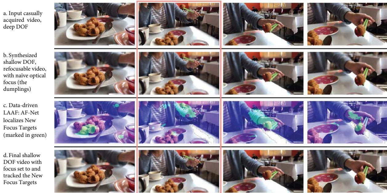
Figure 5.9: Data-driven AF-Net to predict New Focus Targets for video autofocus. (Row 1) Input video shows a dumpling is picked up from the plate. (Row 2) naïve synthetic SDOF video would easily suffer from mis-focus when applied shallow DOF. (Row 3) Focus region prediction from AF-Net; green marks focus with higher probability. Second frame (bounded by red) is the predicted temporal position of the New Focus Target, when the person picks up the dumpling. (Row 4) The resulting video shows autofocus that tracks accurately on the dumpling. Video result can be found in the accompanying video.
