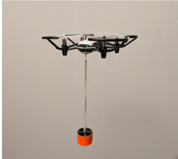
Figure 4.1: DJI Tello with suspended payload.
