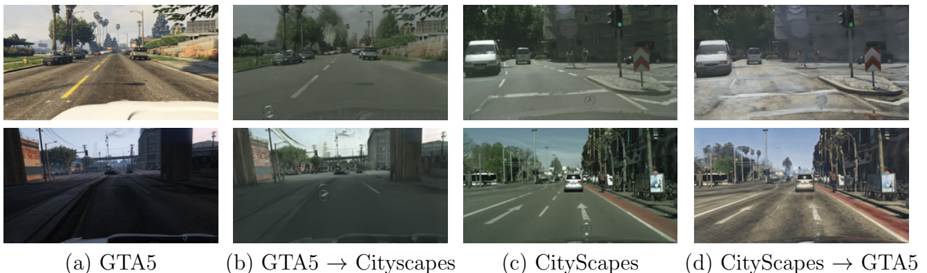
Figure 5.7: GTA5 to CityScapes Image Translation. Example images from the GTA5 (a) and Cityscapes (c) datasets, alongside their image-space conversions to the opposite domain, (b) and (d), respectively. Our model achieves highly realistic domain conversions.
