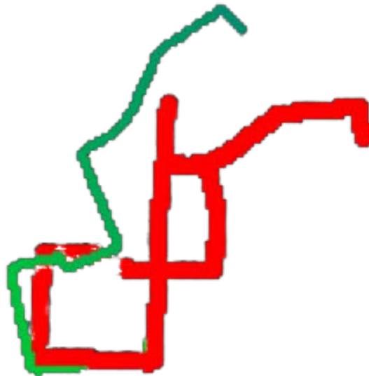
Figure 4.3: Trajectory of FAST without dynamic thresholding on sequence 0 when 0 mean gaussian noise with a standard deviation of 60 is added to the images. In green is the predicted trajectory, and in red is the ground truth trajectory. FAST is able to closely follow the until about halfway, where it misses a turn and diverges.
