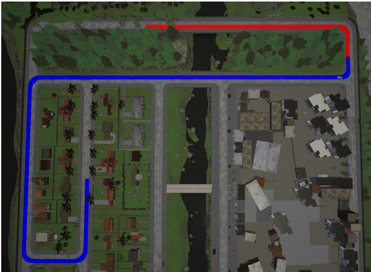
Figure 3.2: A* Route planning over the road graph in Carla. This search takes into account the driving direction of the lane, but does not consider static or dynamic obstacles. The nodes in the road graph are coarsely spaced waypoints on the road and the lanes are connections between these waypoints. Here red indicates the path that has already been covered by the ego-vehicle, while blue represents the path that has yet to be covered.
