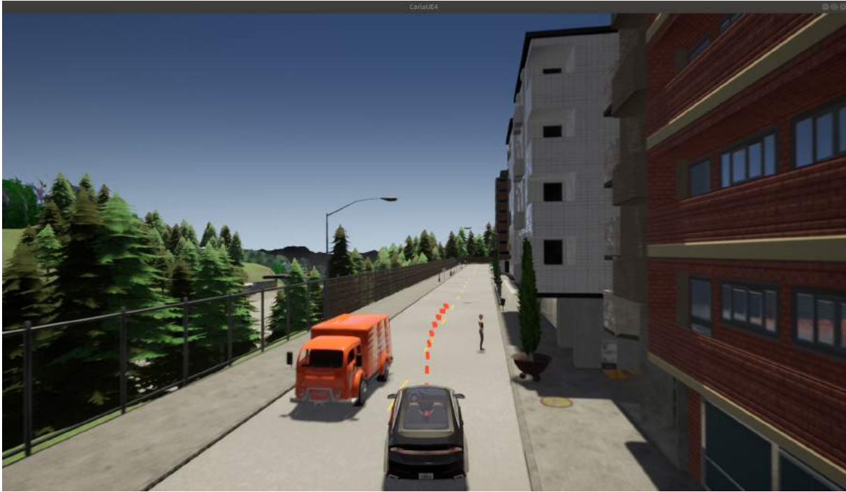
Figure 5.3: Person Behind Car scenario. The ego-vehicle must successfully navigate between a tight space formed by the red truck and pedestrian.
