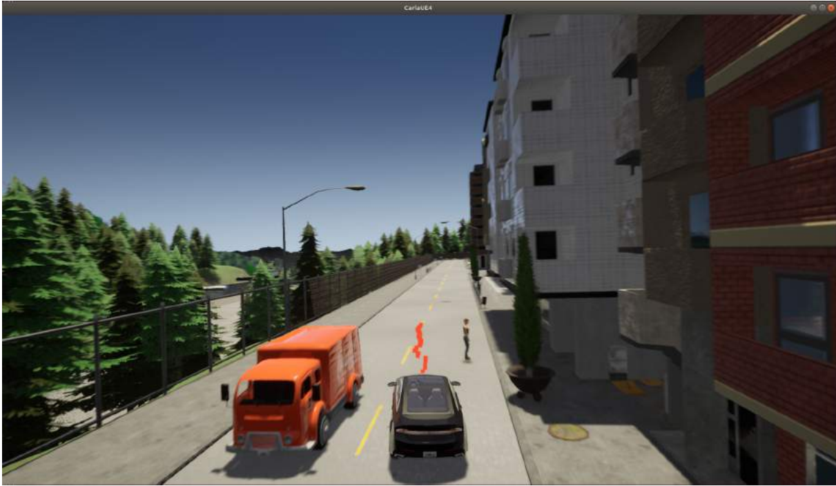
Figure 6.14: Visualization of the RRT* planner in the pedestrian behind car scenario
