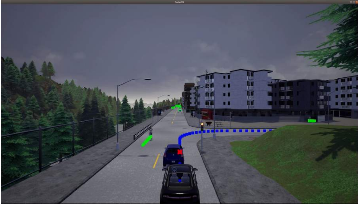
Figure 3.4: Planning and prediction in Carla. Here we visualize our planning and prediction modules in the Carla simulator. In this scenario, the ego-vehicle should follow the global route indicated by the blue points. Green points represent predicted trajectories of other agents. We note that the ego-vehicle is stopped behind a car at a red light. The motion planner must account for the global route, dynamic obstacles and traffic state to safely produce a motion plan.
