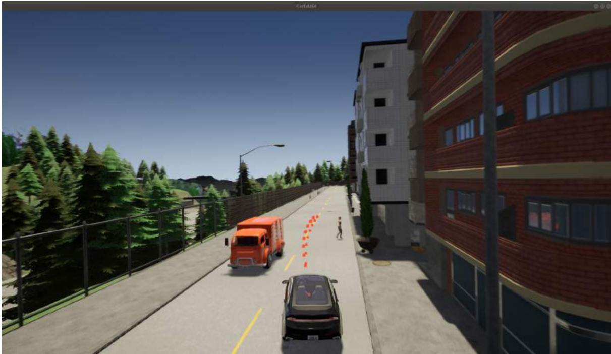
Figure 6.9: Visualization of the Frenet Optimal Trajectory planner in the Carla pedestrian behind car scenario.
