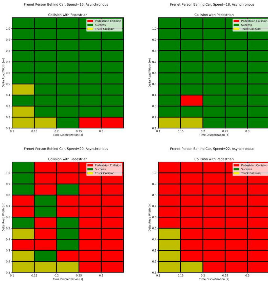
Figure 6.3: Frenet Optimal Trajectory collision tables for asynchronous cases.
