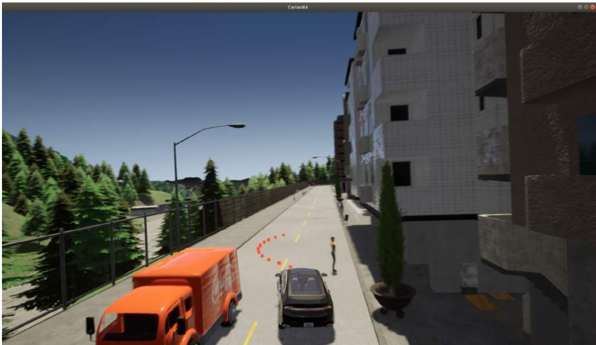
Figure 6.18: Visualization of the Hybrid A* planner in the pedestrian behind car scenario.
