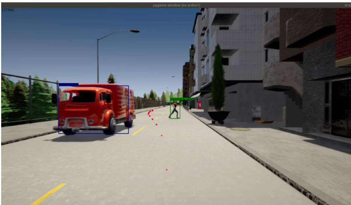
Figure 2.3: Object detection in Carla. Here we visualize our pipeline running end-to-end in Carla. On screen we visualize the Faster R-CNN [57] bounding box predictions from a first person perspective. Faster R-CNN successfully identifies the truck and pedestrian in this scenario. This information is used by motion planning to produce a safe trajectory between the obstacles. The trajectory is shown as red points.
