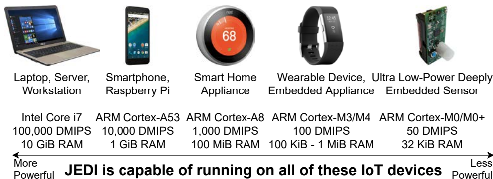
Figure 4: IoT comprises a diverse set of devices, which span more than four orders of magnitude of computing power (estimated in Dhrystone MIPS). 1
