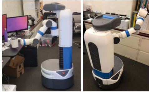
Figure 4.4: A Fetch robot performing two decluttering tasks in the experiments. As the robot approaches a desk (left) and a bookshelf (right) it computes a road map of motions for its 8-DOF manipulator arm using serverless computing, it then uses to perform a sequence of decluttering tasks.
