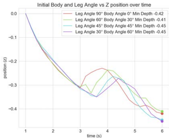
(c) Variations in initial body and leg angles have similar effects as varying leg angles only
