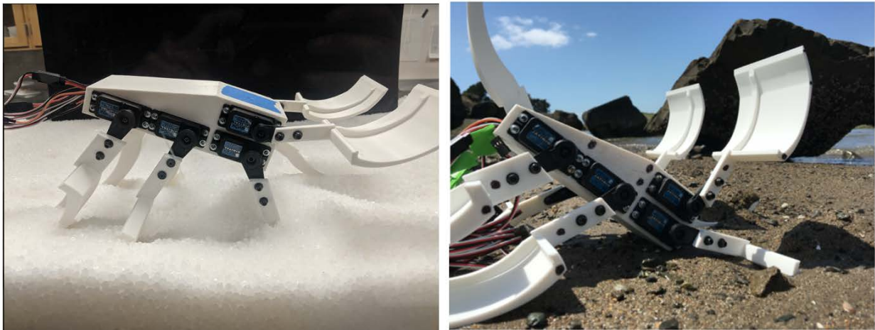
Figure 3.3: 3D printed physical robot with 1DOF G1 and G2 limbs, Left: Subject in test bed
