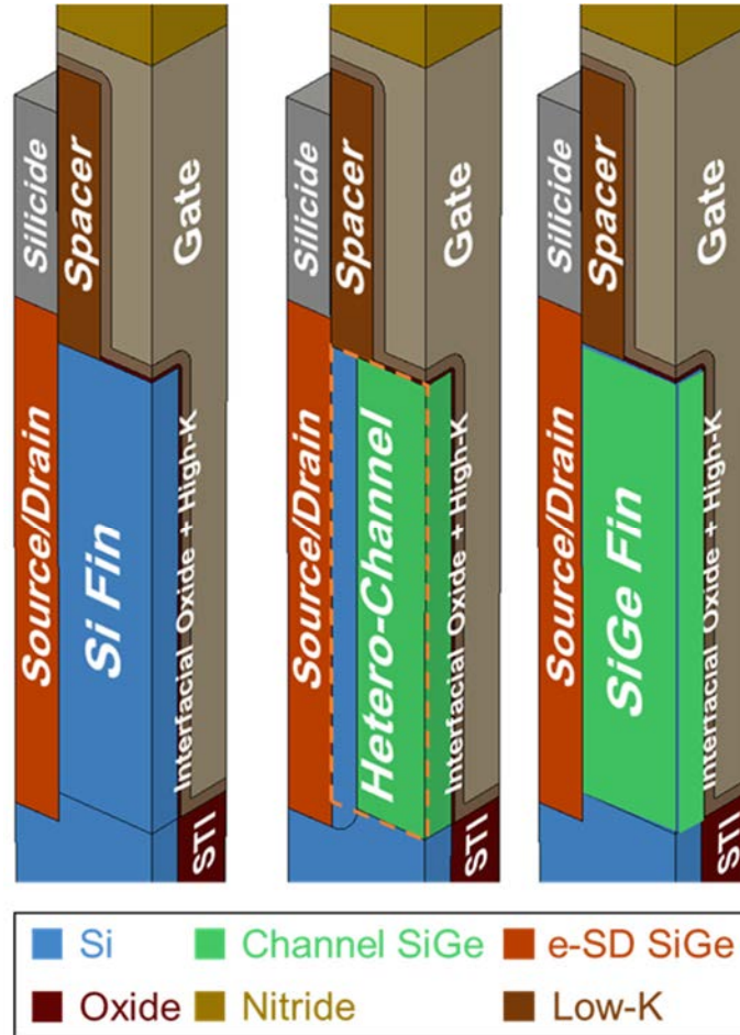
Figure 2.1-1. Double cutaway views of the two transistor structures studied in this work. (Left: Control Si FinFET, middle: Hetero-Channel FinFET, right: Control SiGe FinFET). The dashed lines circumscribe the hetero-channel. Different colors are used for the \text{Si}_{1-x}\text{Ge}_x in the channel region vs. the \text{Si}_{1-y}\text{Ge}_y in the embedded source and drain regions, to denote different Ge mole fractions. In this work, \text{Si}_{0.5}\text{Ge}_{0.5} is used for the source/drain contact regions. The fin height is defined to be the height of the fin above the shallow trench isolation (STI). L_{\text{eff}} , the effective channel length, is defined to be the lateral distance between the locations where the S/D dopant concentration falls to 2 \times 10^{19} \text{ cm}^{-3} .
