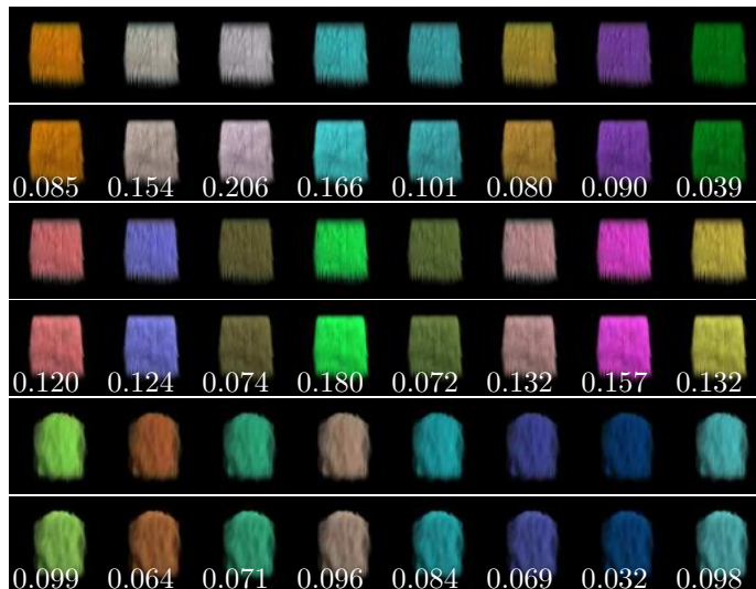
Figure 4.41: Validation of our neural network training. Odd numbered rows are rendered with path tracing of actual hair/fur fibers as reference. Even numbered rows are rendered using best fitted/predicted parameters as BSSRDF. Top two rows: selected training set and fitting. Middle two rows: selected test set with same geometry but different lighting conditions. Bottom two rows: selected test set on another scene. Our trained neural network predicts a perceptually similar match, compared to the reference. The numbers in the figures show the loss value of each fitted image. Recall that the loss function is defined in Section 4.12.
